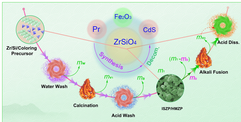
Figure 6 Chart of the mass divergence of a chromophoric element throughout the process from synthesis to decomposition and to the dissolution of the zircon pigments
